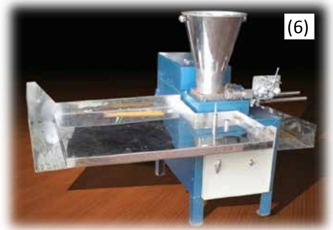
Figure 13. Series of bamboo processing machines for incense stick: 1) cutting machines, 2) bamboo splitting, star blade, 3) bamboo thinner, 4) bamboo stick slicer, 5) polish and 6) incense machine.
